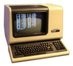
Your terminal window is just a software version of this old appliance. You will enter commands into this window to get the remote machine you are communicating with to perform various tasks.
